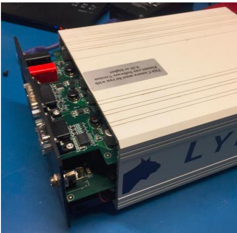
**Step 3:** Remove four (4) screws from the Heat Sink Plate. Remove the plate.
