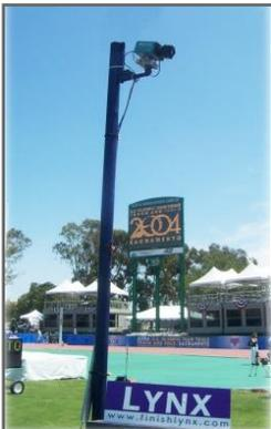
Because finish line cameras are often mounted well above eye-level, the **Remote Lens** and **Remote Positioner** upgrades ensure the camera is easily accessible and adjustable. These motorized accessories allow operators to make mid-meet adjustments quickly and easily to account for changes in glare, shadows, or camera positioning. A simple click on the remote icons will adjust the lens or field-of-view without having to climb a ladder to reach the camera.
