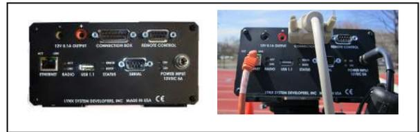
3. Connect the female end of connection cable to the port on the back of the camera labeled **Connection Box** and the round metal XLR end to the 500' Start Sensor cable.
