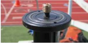
4. Secure the geared head to the stud on top of the tripod.
