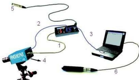
1. Connect the female end of connection box cable to the port on the back of the camera labeled **Connection Box** and the male end to the left side of the connection box.
