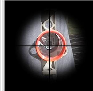
4. When the LaserLynx prism is at the center of the crosshairs, the operator taps the **acquire** button on the FieldLynx unit and distance is calculated.
