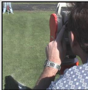
3. Using the built in telescopic sight, the LaserLynx operator aligns the unit on the prism held by the marking official.
