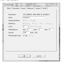
c) Click on the Parameters tab and set the Frame Rate and Density to your desired need. If you see any problems with image capture, lower the frame rate, and/or return the Pixel Mode to Wide 50%.
