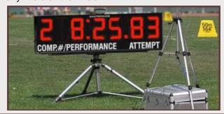
**SeriaLynx** enables fast and secure wireless communication between the FieldLynx netbooks and the LED display/wind gauge. One unit connects to the LED display to show live marks and standings from FieldLynx while the other connects to the wind gauge to wirelessly pull live wind readings for jumping events.
